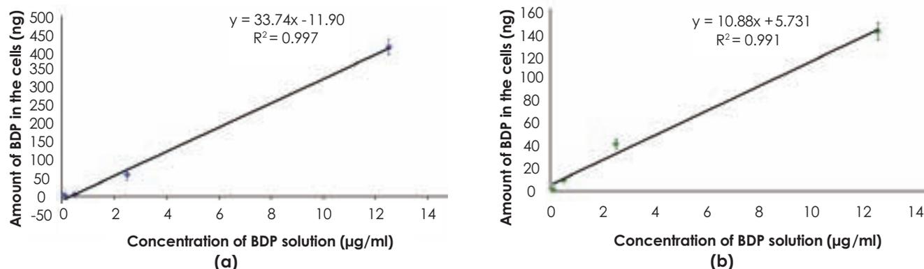
increases linearly with that of the added BDP solution (Fig. 2b).
