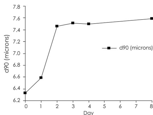
**(b) Particle size (d90) (■) over time after single pass micronization.**
