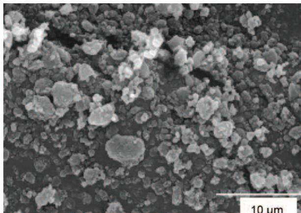
**(a)** FP micronized by conventional air jet milling.
