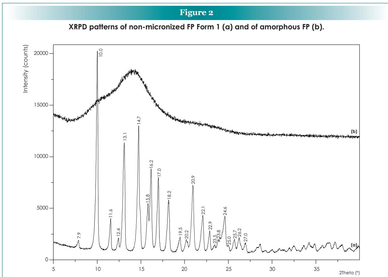
amorphous material,\*, for samples left at room conditions, was measured as a function of time. Simultaneously, water content and particle size analyses were executed. With time, conversion to crystalline form occurred and, in four days, the amorphous content decreased from 47% (w/w) to 8.7% (w/w). In conjunction with this decrease, water content decreased (the amorphous form is more hygroscopic) and particle size increased.
