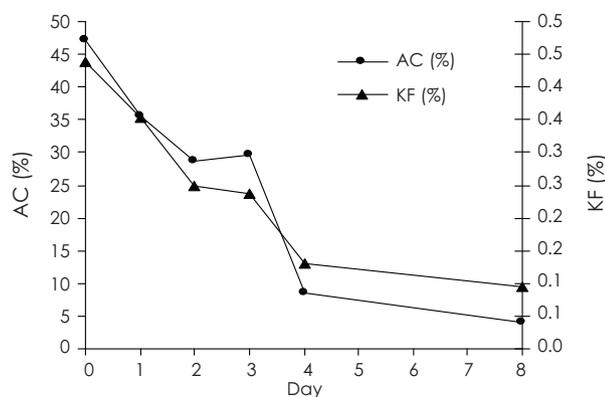
**(a) Amorphous (●) and water (▲) content over time after single pass micronization.**
