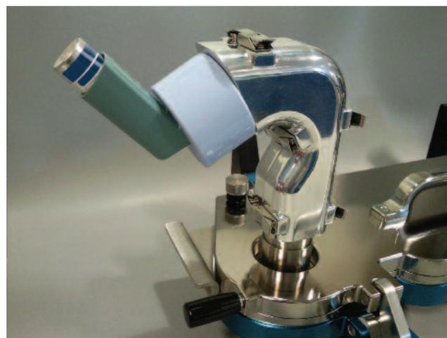
maceutical ingredient(s) of the product. Typically, it involves either an Andersen Cascade Impactor (ACI) or Next Generation Impactor (NGI) with the USP/Ph.Eur. induction port being the standard interface physically connecting the inhaler with the CI. Its purpose in the compendial methods is to provide a uniform and robust representation of the human throat and upper airway for testing purposes in the context of product quality control.
