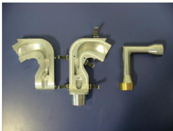
Precision manufactured to close tolerances; the AIT has a highly reproducible, human-like geometry and delivers flow-rate-independent performance.<sup>8</sup> In experiments with both pressurized metered dose inhaler (pMDI) and dry powder inhaler (DPI) formats, undertaken during its development,<sup>6</sup> the AIT collected more of the emitted
