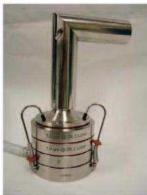
FSA with 1.0 and 5.0  $\mu\text{m}$  stage cut-point sizes
