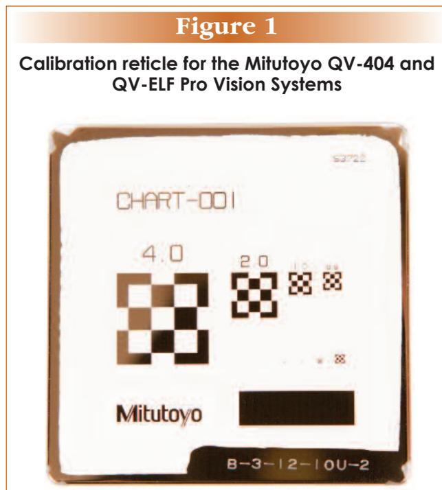
The calibration reticle that MSP employs has all-square features with dimensions ranging from 20 microns to 4,000 microns. These dimensions are determined every five years with NIST-traceable laser interferometry at a local laboratory, yielding accurate values to within 0.6 micron (95% confidence interval).
