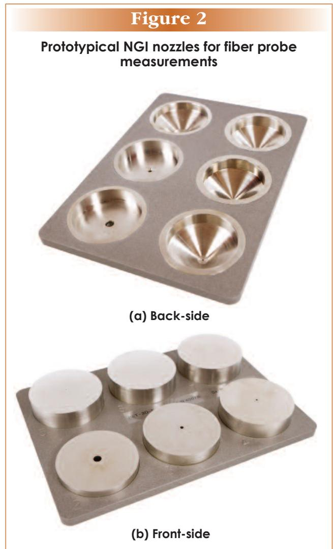
nozzles at several locations *inside* the nozzles, mapping the nozzle shape by physical touch of the fiber probe to the wall of the nozzles, contacting 48 touch points around the nozzle circumference and repeating these measurements 10 times at each depth position. In this way, the fiber touch probe method gives a true physical measurement of the coordinates of the inner wall of each nozzle so examined, leading immediately to a least-square calculation of circumference, diameter and area.
