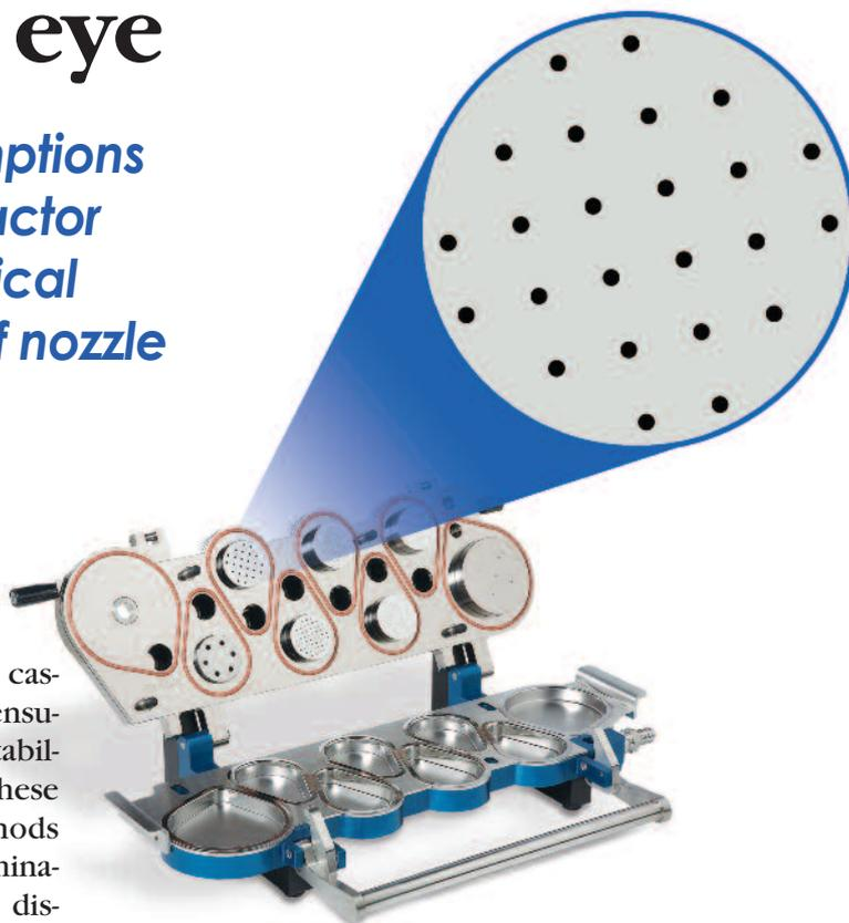
nozzle measurements are important because impactor nozzle specifications for new and used impactors hinge on single-digit micron boundaries. If the object studied is not round, then “diameter” begins to lose its meaning as a single-parameter method of quantifying nozzle dimensions. Indeed, the pharmacopeial specifications for impactor nozzles presume roundness but with no definition of its meaning. The following discussion explains a path forward for remedying this oversight.
