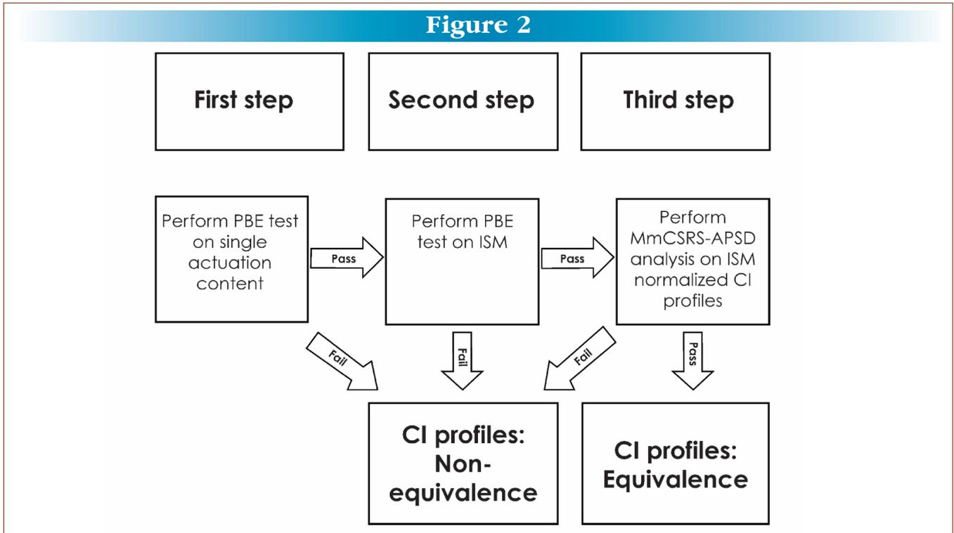
Flow chart of the proposed stepwise cascade impactor equivalence test. ISM: impactor sized mass. This flow chart was previously published in Weber B, Lee SL, Delvadia R, Lionberger R, Li BV, Tsong Y, et al. Application of the modified chi-square ratio statistic in a stepwise procedure for cascade impactor equivalence testing. The AAPS Journal. 2015;17(2):370-9.
