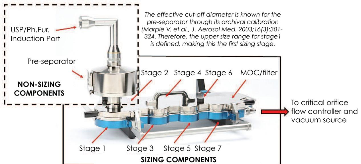
The NGI in setups for testing pressurized metered dose inhalers (pMDIs) and dry powder inhalers (DPIs), including categorization of NGI stages into size measurement and non-size measurement components.
