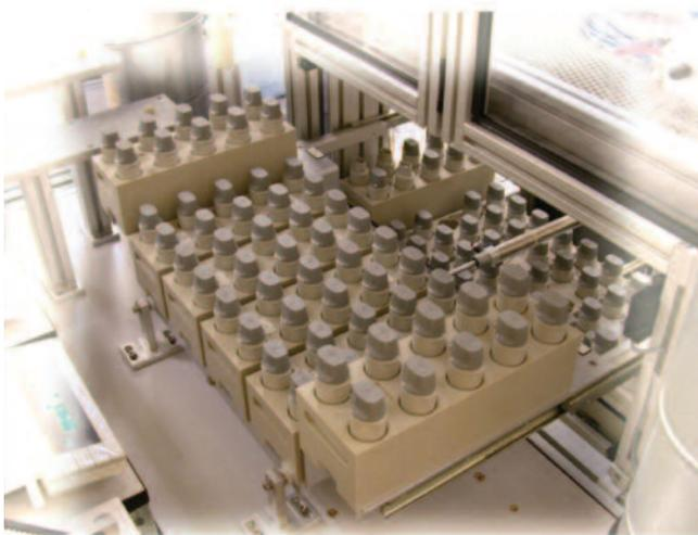
A set of trays giving access to 60 inhalers. In total, five similar racks can be program-selected, providing storage capacity for 300 devices.
