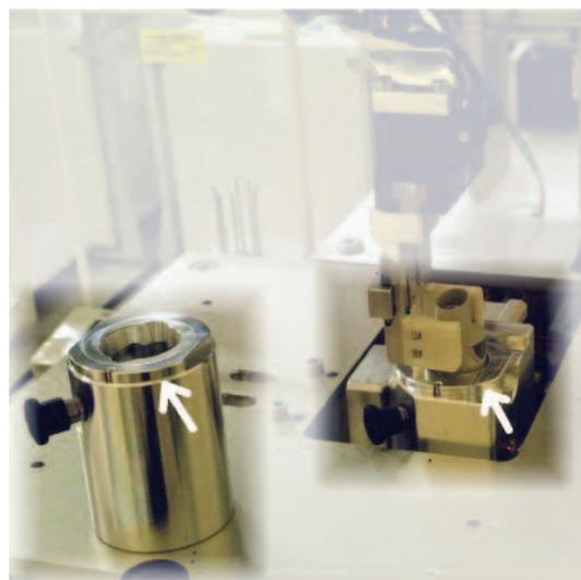
Figure 3 shows an example of the modular design of the sample interface. Inserts in the different stations allow for a quick change thereby enabling design modifications of the device under test. The gripper unit of the robotic arm was first designed using metal tweezers but later molded-fiber-enforced epoxy grippers were used. Finally, the grippers were made of three-dimensional rapid prototypes and provided such a good hold that spring-loaded, pre-determined breaking points were installed.
