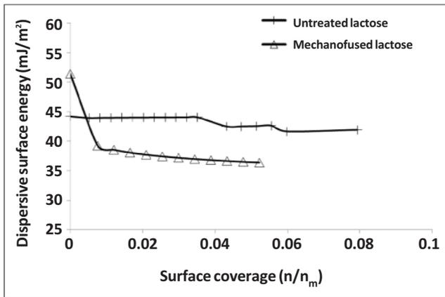
Figure 2. Only less than 1% of the mechanofused lactose particle surface has high dispersive energy; more than 99% of the surface has a lower dispersive energy than that of the milled lactose powder. Reprint from reference 32 with permission from John Wiley and Sons.
