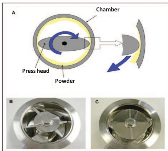
Figure 1. (A) Diagram of dry coating process; (B) Image of mechanofusion AMS-Mini system with a Nobilta processor; (C) Image of mechanofusion AMS-Mini system with a Nanocular processor. Figures B and C are reprinted from reference 29 with permission from Elsevier.
