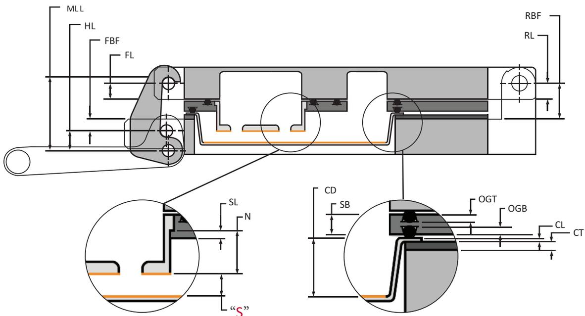
This figure displays the individual dimensions that together define the distance “S” from the nozzle exit plane to the cup collection surface. The value of “S” can be calculated from the rear hinge pins or from the front hinge pins.
