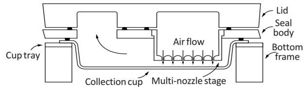
This multipoint inspection ensures cup flatness, at the same time ensuring proper cup depth across the critical region where particles are deposited. The thoughtful user knows that it is insufficient for the cup to satisfy the depth specification *on average*. That is because a cup could, in principle, have an *in spec* average depth *but at the same time have every single measured depth out of specification*.
