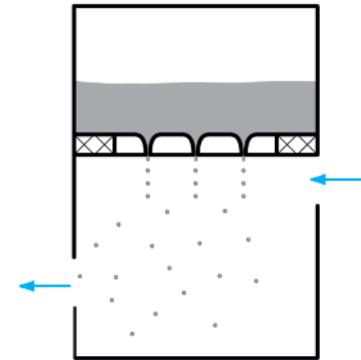
Aerosol generated when columns of fluid are extruded from small mesh holes and break up to form aerosol droplets; droplet size is related to hole size; droplets exit the nebulizer for inhalation.
