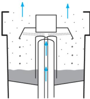
Aerosol generated by the breakup of a fast moving air/liquid mixture; larger droplets impact on baffles and are returned to the bulk fluid; smaller droplets exit the nebulizer for inhalation.
