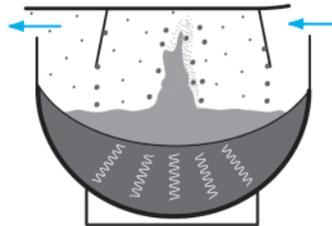
Aerosol generated at the peak of a fountain created by focused ultrasonic waves; larger droplets impact on baffles and are returned to the bulk fluid; smaller droplets exit the nebulizer for inhalation.
