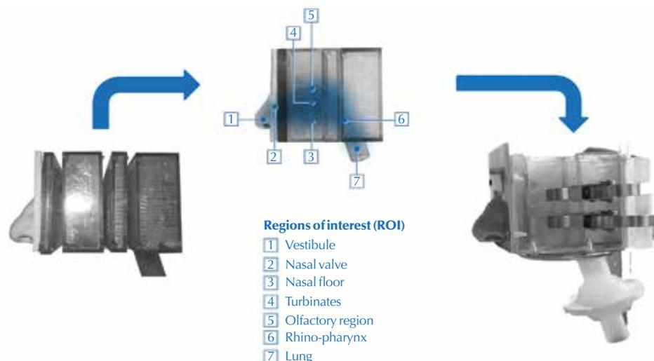
using *in vitro* nasal deposition study in a physical airway nasal model with identical dimensions and geometry to the computational model.<sup>41</sup>
