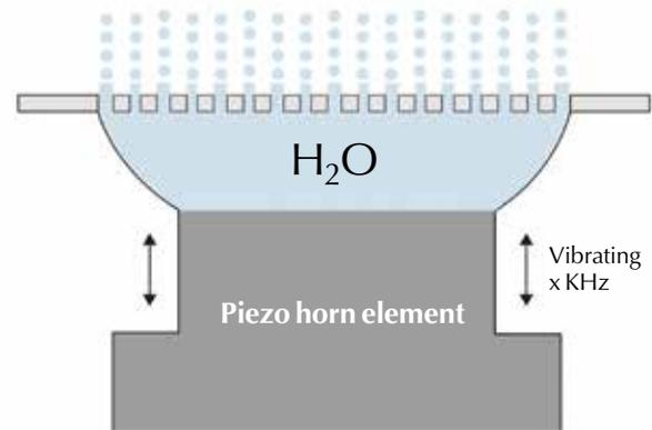
the mesh (Figure 13). The configuration is also preferably circular. This technology has been implemented in conventional and small handheld nebulizers.<sup>30</sup>
