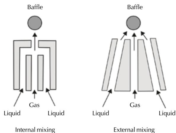
lets are transported to the nebulizer outlet (and the patient). More than 99% of the aerosol produced is returned to the reservoir; only about 1% reaches the nebulizer outlet.<sup>17,18</sup> The nebulizer nozzles have two designs; one where the air and liquid are internally mixed then ejected through a secondary orifice and the other that uses an external mixing design where the secondary nozzle is omitted (Figure 4). Both types are frequently seen in various nebulizer brands.
