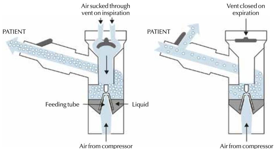
inhales but not when a patient exhales (Figure 6). They are intended to enable more efficient use of the liquid to be aerosolized and can shorten overall treatment time.
