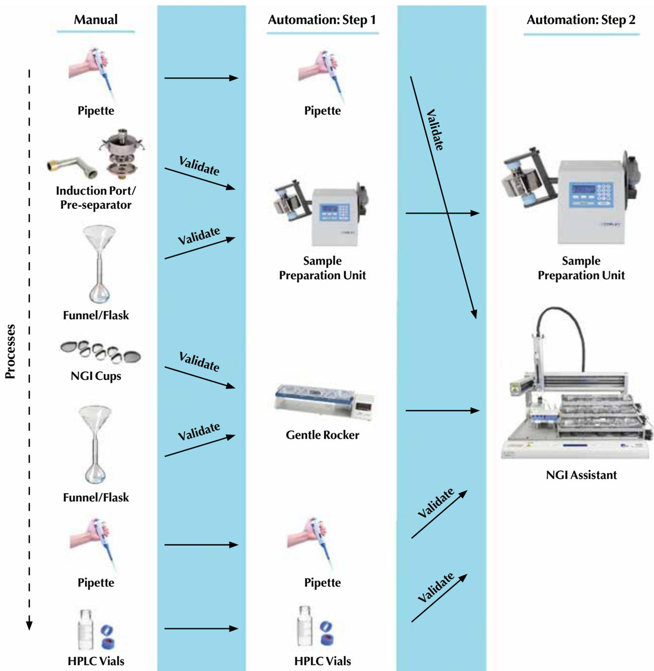
tivity, and the potential for high returns/short payback times, particularly for the routine testing associated with QC. With a stepwise approach, these benefits can be accessed with minimal risk.
