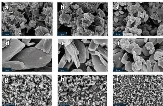
in Figure 3c). Wet polishing produced noticeably smoother-surfaced particles because, in this two-step milling process, the applied energy is highly dispersed in the liquid, thereby decreasing stress in the particles and producing polished surfaces.
