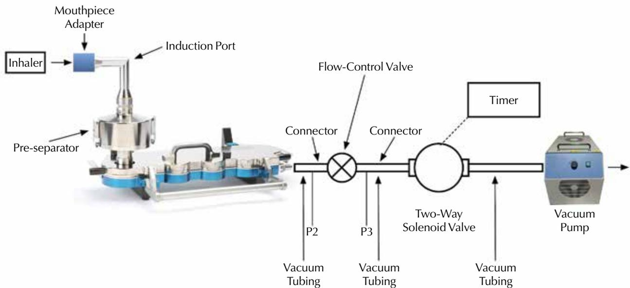
number of seconds at a target flow rate when it is attached to a good-quality cascade impactor (Figure 1). This figure calls out common test components described in USP Chapter <601> [5] and in Pharm. Eur. Section 2.9.18 [6].
